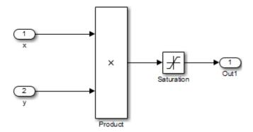
The Simulink Design Verifier software generates errors when attempting to satisfy the upper and lower limits of the Saturation block, because the software does not support nonlinear arithmetic. To work around these errors, restrict one of the inputs to a set of discrete values.
