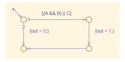
Given that A, B, and C are all separate inputs, there are five possible ways to evaluate the condition on the Stateflow transition, shown in the following table.
