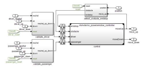
The  ${\tt control}\ Model\ block\ references\ the\ {\tt slvnvdemo\_powerwindow\_controller}\ model.$
