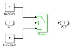
The Switch block is outlined in green, which indicates that the Switch block has test cases that satisfy its test objectives.
