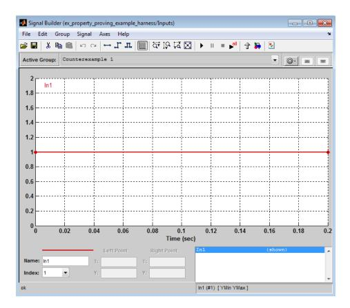
The input signal 1 causes the output of the Compare to Zero block to be 0. This counterexample violates the proof objective that specifies that the output of the Compare to Zero block be 1.
