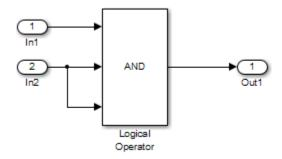
When the Simulink Design Verifier software analyzes this model for Condition Decision coverage, the analysis can only satisfy five of six objectives for the Logical Operator block inputs. The software cannot generate a test case when the third input to the Logical Operator block is false. If the second input is false, the third input is false, but the software ignores the third input due to the short-circuiting. If the second input is true, the third input is never false.
