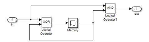
The persistent information in this model is limited to the Boolean value of the Memory block. The input to the model is a single Boolean value. The following table describes the complete behavior of the model, including the behavior that would result from an arbitrarily long sequence of inputs.
