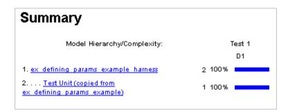
This section summarizes the coverage results for the harness model and its Test Unit subsystem. Observe that the subsystem achieves 100% decision coverage.
