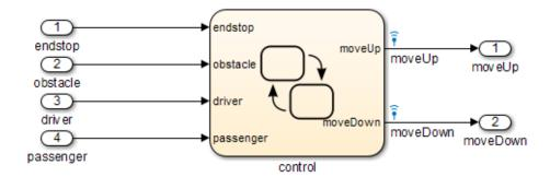
The referenced model contains a Stateflow chart control, which implements the logic for the power window controller.
