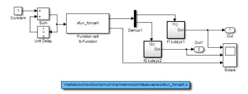
The Simulink Design Verifier software does not support the S-Function block, so if automatic stubbing is enabled, the analysis ignores the behavior of the S-function. As a result, the code that triggers the two function-call subsystems is ignored, resulting in two unsatisfiable objectives. Since the function calls are ignored, the contents of those subsystems are effectively eliminated from the analysis.
