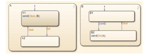
If you change the send function calls to use directed event broadcasts so that the Set and Clear events are broadcast directly to the states B1 and A1, respectively, the cyclic behavior disappears and the Simulink Design Verifier software can analyze the model.
