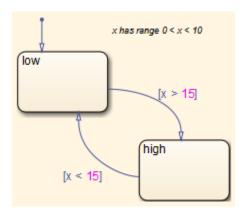
The value of x must fall between 0 and 10, so the transition condition [x > 15] is never true. The transition from low to high never occurs. Because the high state is never entered, the transition condition [x < 15] is never tested, and the transition from high to low never occurs; the chart is always in the low state.
