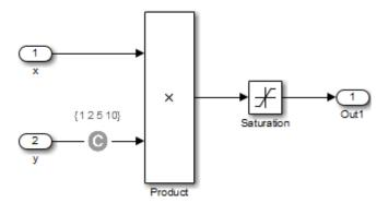
You can also constrain signals that are intermediate or output values of the model. Constraining such signals makes it easier to work around multiplication or division inside lower level subsystems that do not depend on model inputs.
