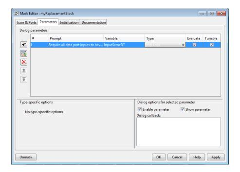
**Note** When you create mask parameters that control the behavior of parameters associated with their underlying blocks, specify actual parameter names as dialog box variables in the Mask Editor. For instance, InputSameDT is the actual parameter name that controls the Require all data port inputs to have the same data type parameter of the Multiport Switch block; therefore, it specifies the name of the dialog box variable in this example.
