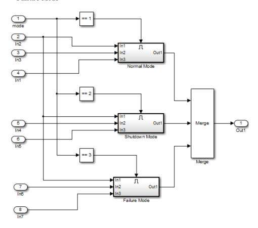
You can incrementally generate test cases for each subsystem by constraining the first input to a constant value before running an analysis. In this way, as you create test cases for each subsystem, the software ignores the complexity of the other two subsystems.
