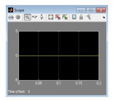
The Scope block displays the value of the signal output by the Compare To Zero block in your model. In this example, the Compare To Zero block returns 0 (false) throughout the simulation, which falsifies the proof objective that the output of the Compare to Zero block be 1 (true). The counterexample that the Signal Builder block supplies falsifies the proof objective.
