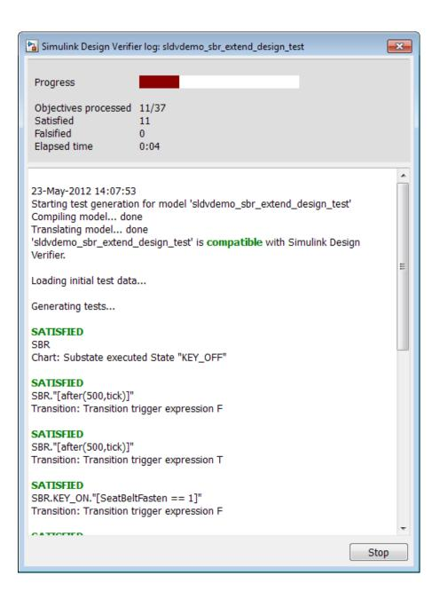
The log window then lists the objectives generated beyond the starting test case.
