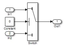
For this Switch block, the control input is always 0. If the **Criteria for passing first input** block parameter is u2 ~= 0, the Switch block always passes the third input through to the output port. When you analyze this model, the Simulink Design Verifier software removes the Switch block from the model and does not report any test objectives for the Switch block.
